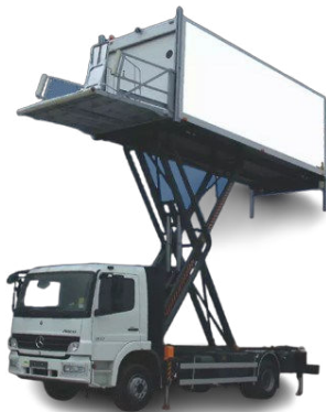
AST.CT 5800 Main Deck Catering
